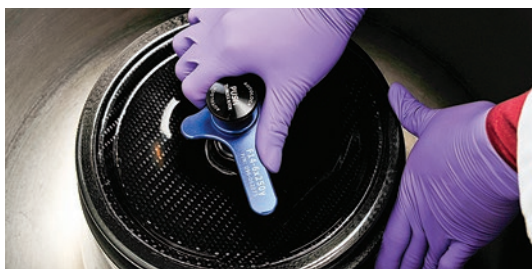
Innovative speed handles make tightening the lid safer while also simplifying lid removal
